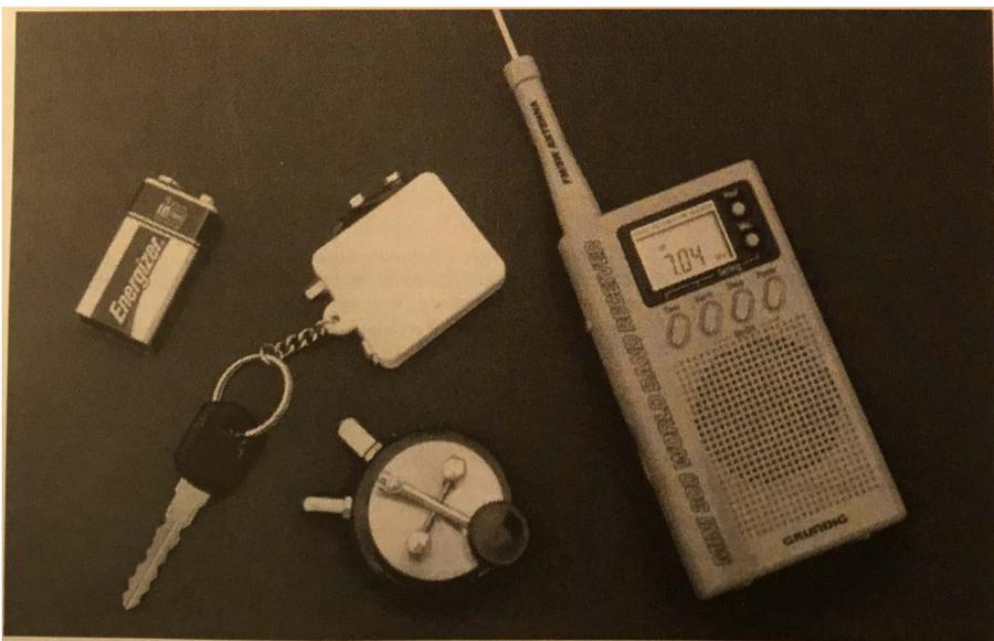
**Photo 3** When placed beside a low cost AM type shortwave receiver, the mini project serves as a wireless BFO for receiving CW signals. Two adjacent frequencies are switch selectable without retuning receiver and transmitting back to stations simply involves tapping Morse code with the key. A slight CW offset is also included. Details in text.
