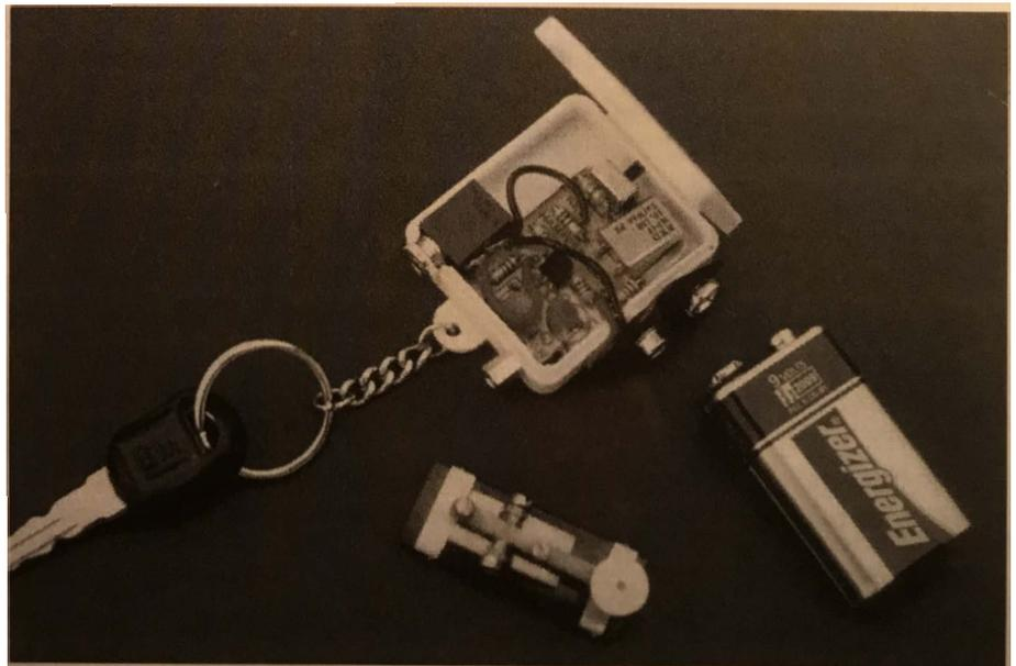
**Photo 2** The completed four function mini project mounted in a tiny keyfob pillbox for "go anywhere HFing" Just add a 9V battery, miniature Morse key and dangling wire antenna and you have the ideal travel mate
