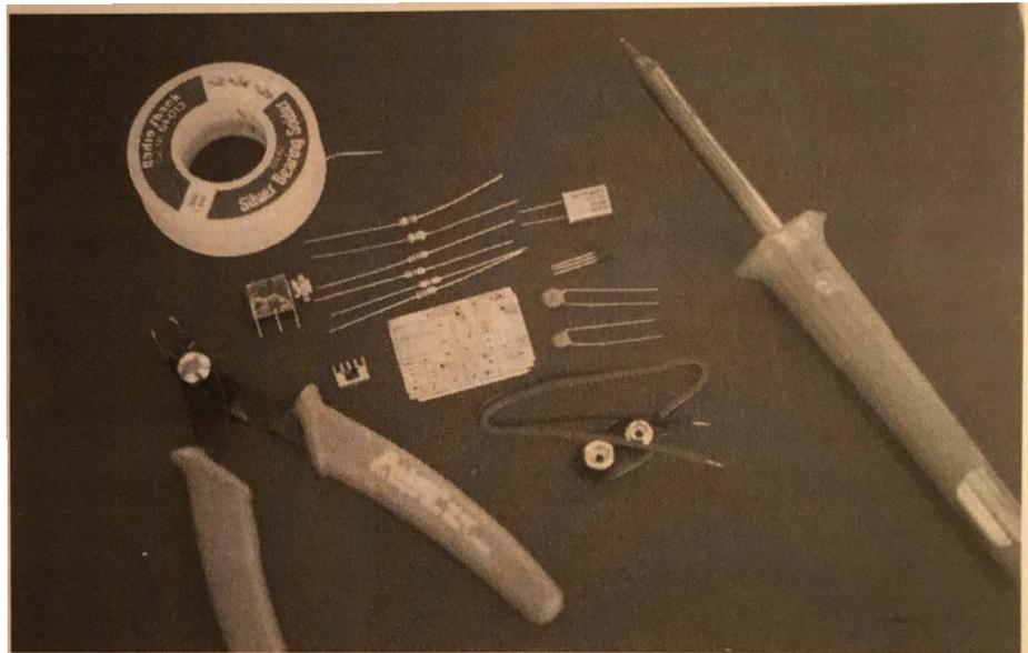
**Photo 1:** Our featured mini-project laid out and ready for assembly. This little gem consists of only 12 parts yet it is a combination QRP transmitter, wireless BFO/receive converter, personal emergency beacon and low gain micro transceiver on a 1 x 1.5 inch (25 x 38 mm) PC board. It is an ideal "first project" for new homebrewers.
