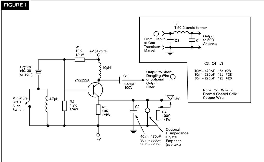
Figure 1: Circuit diagram of the One Transistor Marvel with inset showing values of optional band filters. Data in text.
